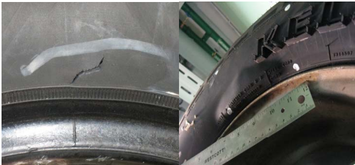
Crack and Bulge
